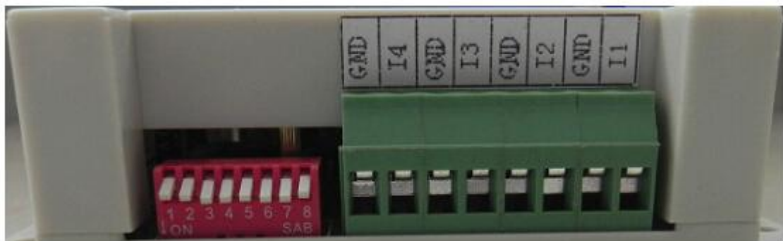
Pic 2: Switch input wiring terminal schematic
